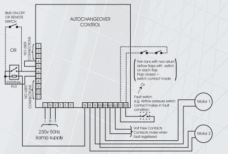
Suitable overload protection for each motor and local isolators should be provided by others
