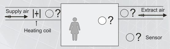
If the supply is for "make up" air, with background heating in the area being served, then a duct sensor should be used. The sensor must be mounted in the supply duct away from direct radiated heat.
